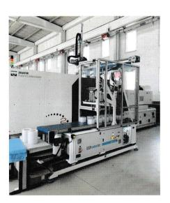
The new Roboter T - Series robot range is designed for IML – In Mould Labeling, insert, pick and place applications and for more flexible automations.
